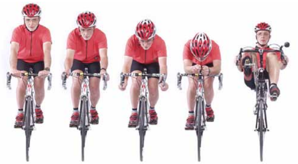
A photographic illustration showing the frontal wind profile of different rider configurations on an upright and recumbent bike.
